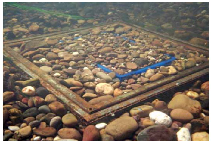
Figure 6: An underwater image of a substrate tray, installed in the River Idle
