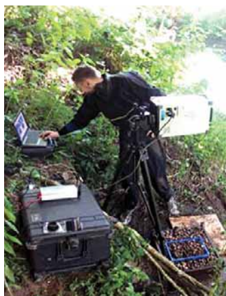
Figure 8: Using the laser scanner to gain Digital Elevation Models (DEMs) of the tray surface.
