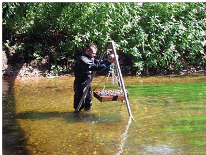
Figure 7: Winching one of the sediment trays from the river bed
